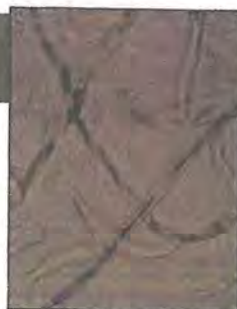
Oil Gator absorbent lint seed magnified 320 times to demonstrate encapsulation of hydrocarbons.
